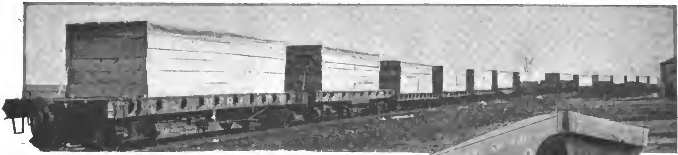
A shipment of fifty-six Chalmers cars to Philadelphia on flat and gondola cars. Two cars go on a freight car. They are well protected with oilcloth and then boxed, the boxes being roofed with waterproof material
